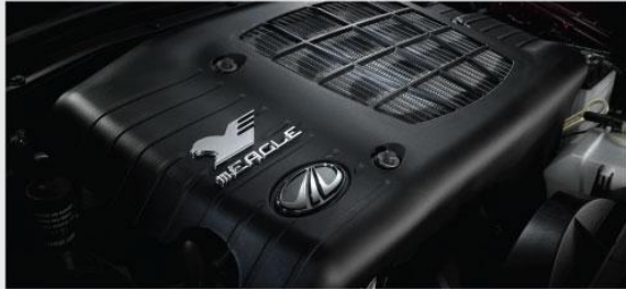
2498cc, 112 bhp mEagle CRDe engine
